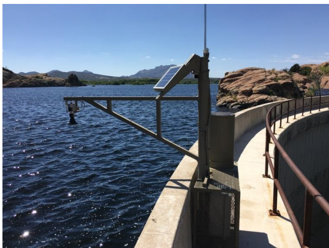
Willow Lake Stage Gage, radar water level. Rain gage and data transmitter located on the dam.
